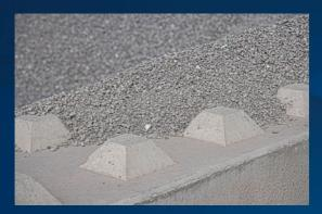
REMEX uses the latest recycling technologies to produce high-quality secondary aggregates from the bottom ash of municipal solid waste incineration plants.
