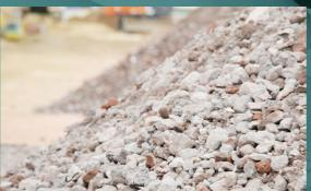
In our recycling plants, the input materials for the production of recycled aggregates are mineral waste from construction and demolition, and road rubble.
